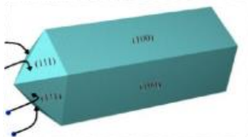
Figure 14: Structure of the five fold twinned nanowire from the work of Yang et Al. 67
