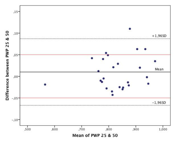
Lines at +0,05 and -0,05: the tolerably small amount that PWP 25 and PWP 50 may differ from each other. Lines at +1,96SD and -1,96SD: limits of agreement. Line at -0,010: mean.
