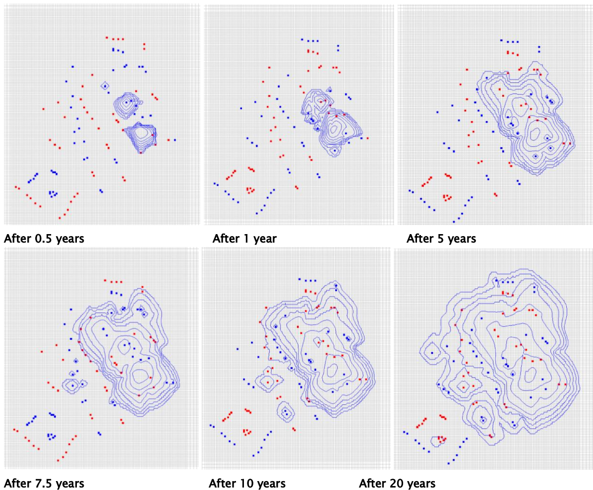
Fig. 25: Contaminant spreading caused by the modeled DNAPL. The contamination contours are logarithmically scaled.
