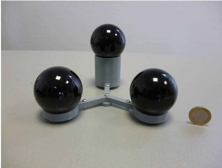
Figure 4: The calibration statue with three spheres and a euro for scale.
