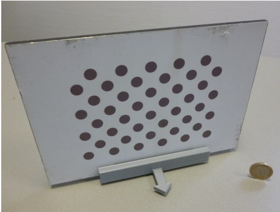
Figure 3: The calibration board used for the calibration of the camera and projector and a euro for scale.
