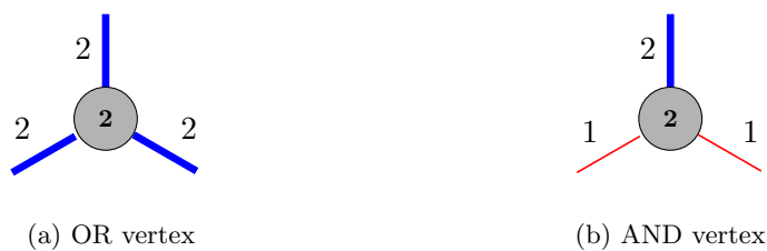
Figure 2.1: The two vertex types from which a restricted constraint graph is constructed: (a) OR vertex and (b) AND vertex. Following the convention set in [1], as a mnemonic weight 2 edges are drawn blue (dark grey) and thick, while weight 1 edges are drawn red (light grey) and thinner.
