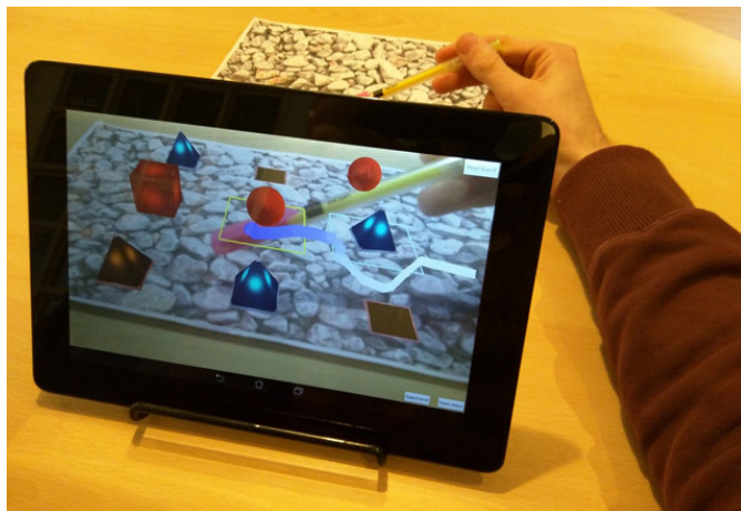
Fig. 1: The created augmented reality game with virtual objects and gesture-based interaction using a colored pen.
