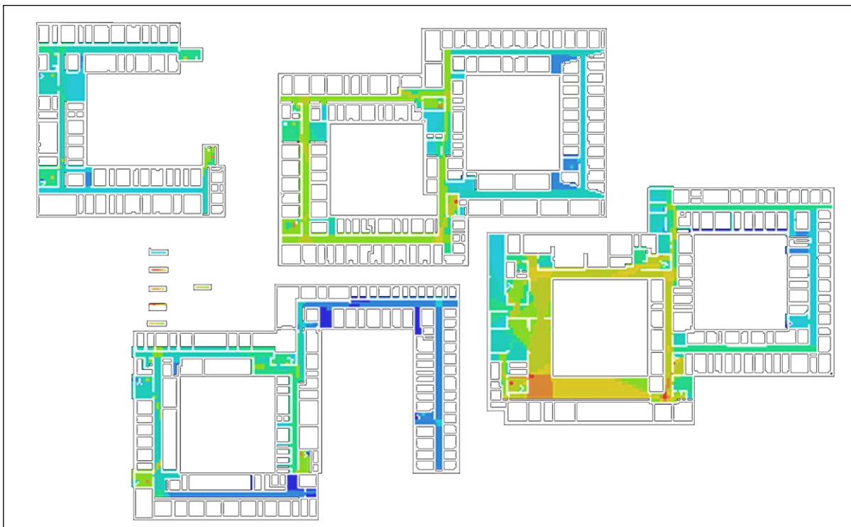
Figure 5: integration scores for the Langeveld building. The Integration score can intuitively be seen as a measure of centrality. A good score is represented by warmer colors (yellow/red), whereas a poor score is represented by cooler colors such as green and blue.
