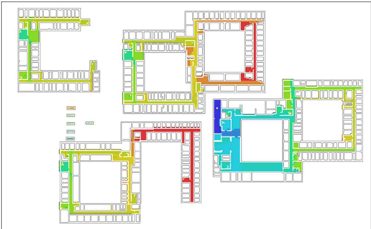
Figure 6: step depth from the main entrance. Higher step depth scores (a high number of visual steps or turns) are represented by warmer colors (yellow/red).
