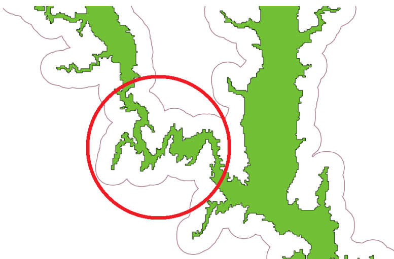
Figure 55: The original polygon in green and the buffer as a solid line around it
