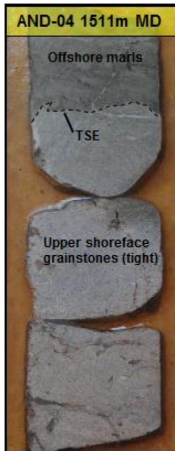
Figure 18. Sharp lithological contact between top ATBR1 (regressive upper shoreface facies) and base ATBRL (transgressive marls, offshore facies), interpreted as a transgressive surface of erosion (TSE). This transgressive surface of erosion marks the top of the ATBR1 formation and represents a sequence boundary.
