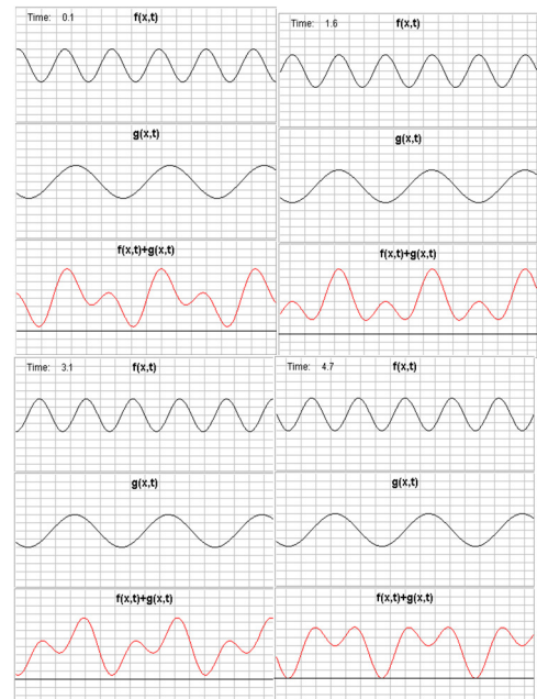
Figure 15 – addition of pure sinusoid functions. Compare the red sinusoids here with the black graphs in figure 14.
