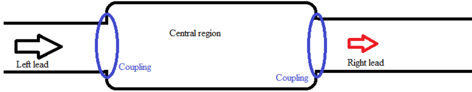
Figure 2.1: A sketch of the assumed setup. All systems are discrete and the leads extend to infinity. A wave enters from the left (black arrow) and we measure the part that is transmitted to infinity through the right lead (red arrow)
