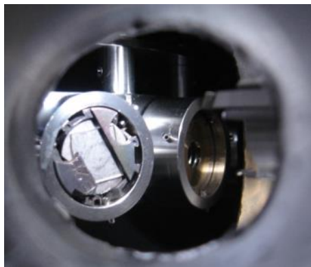
Figure 2.5) The inside of a load chamber where a rectangular-shaped glass sample is held in place by a coin-sized sample-holder inserted in a slot of the carousel. To the right of this slot is an empty slot with no sample-holder.
