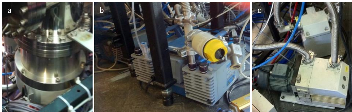
Figure 2.7a) Turbo pump of the Nanocluster source. (b) Diaphragm pumps of load and central chamber. (c) Rotary vane vacuum pump with motor.
