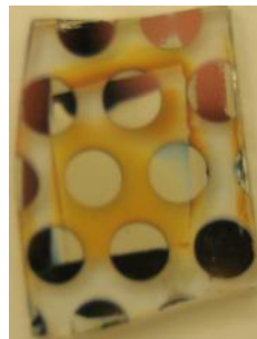
Figure 3.27) Silver conductive layer (white) added to Si layer (yellow) deposited on ITO.
