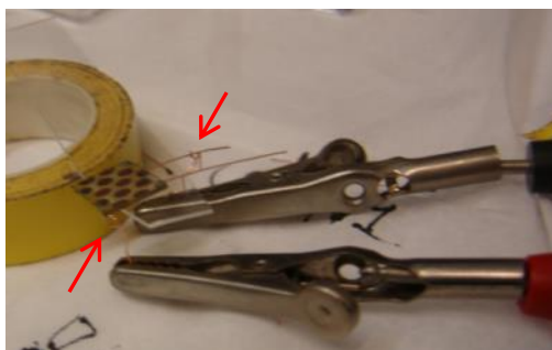
Figure 2.21) Two electrodes measuring the light response from Schottky solar cell. Note that the copper wires held by the alligator clips extend vertically up (red arrows).
