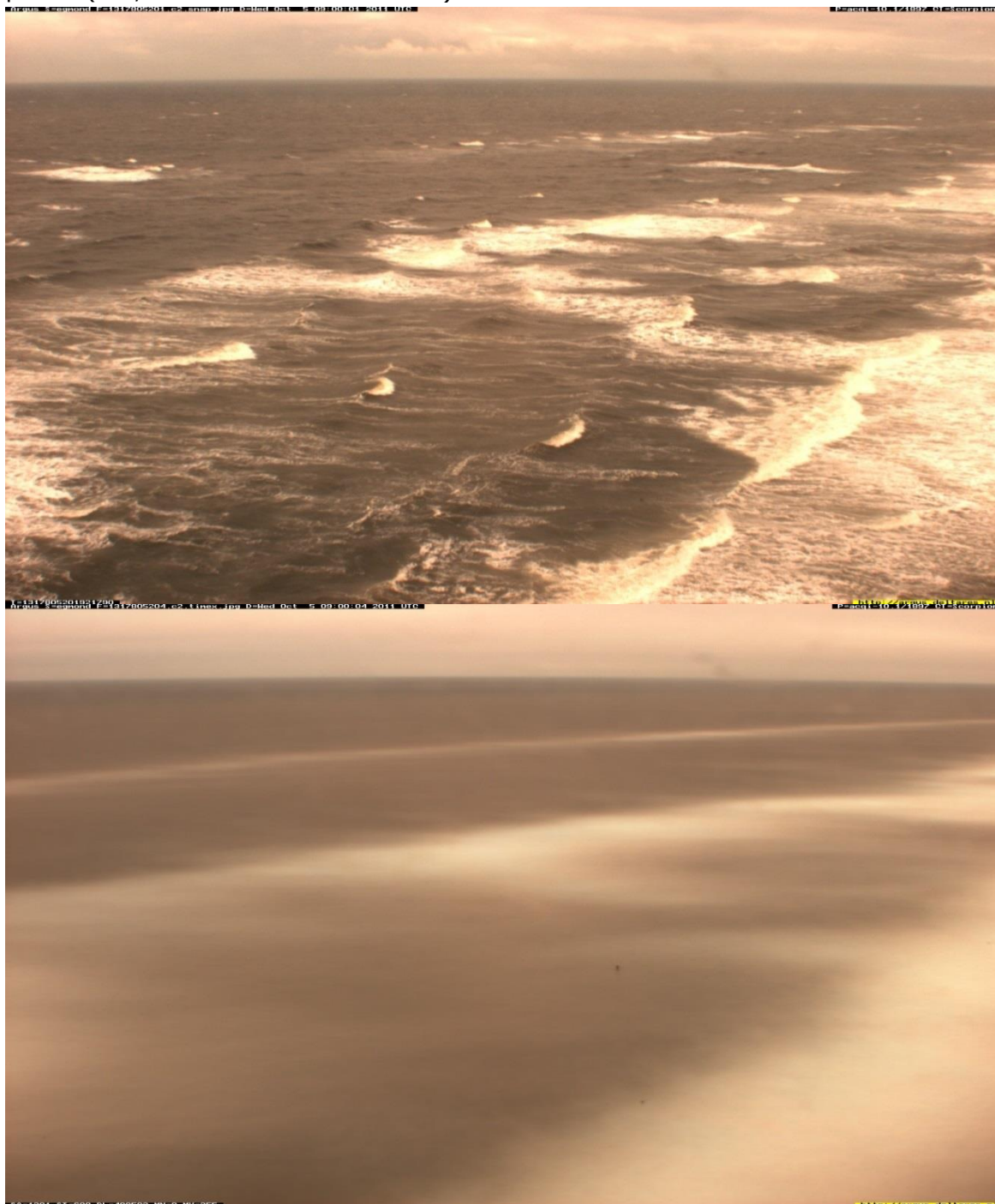
Figure 7. Examples of snapshot (above) and timex (below) images at COAST3D, Egmond, camera 2 for 5 October 09:00:00 GMT.
