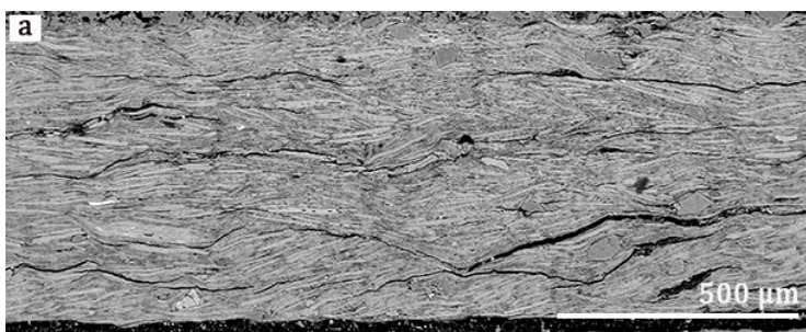
Figure 2.4a) Microstructure of compacted biotite. \sigma_n is ~50 MPa at room temperature (Lu and He, 2014)
