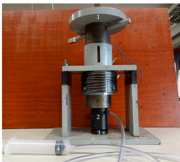
Figure 3.1 An overview of the experimental setup. 1) Weights used to apply the different loads. 2) Delrin POM piston. 3) Delrin POM container in which the sample is placed and loaded 4) Plastic tube connecting Delrin POM piston to either a vacuum pump or a syringe as shown here. 5) Handles used to turn upper piston in shear experiments
