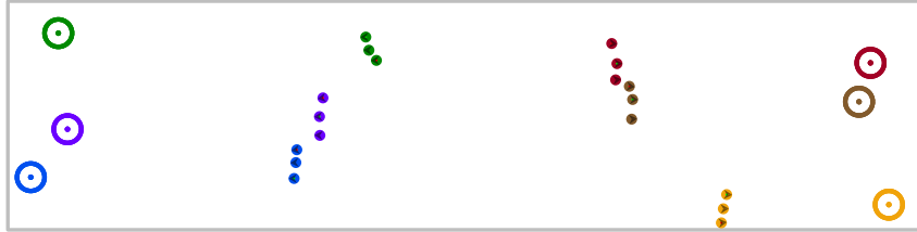
Figure 5.3: Bidirectional-corridor scenario for groups of three: simulation instance using SGN method. For each group, all members share the same color. The goal area of a group is visualized by a ring that shares the color of the group members. A small green ( red ) dot at an agent’s position indicates that the agent currently acts as a leader (last member) of its group, respectively.
