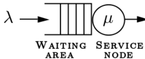
FIGURE 3.1: The M/M/1 queue in graphical notation.
