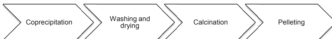
Figure 1.5 Steps in the preparation of the industrial methanol synthesis catalyst
