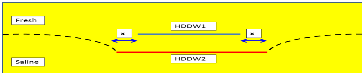
Figure 5.6 - A proposed design modification of the current Freshmaker design: increasing HDDW2 with a length X. This will increase the area over which the fresh-saltwater interface can be lowered.
