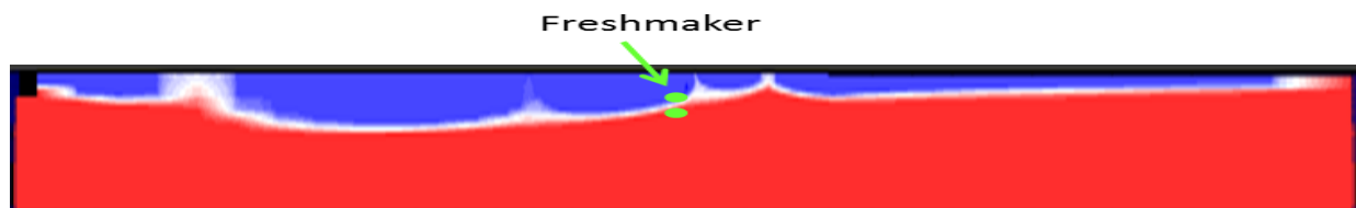
Figure B5 – Initial TDS concentration. Concentrations ranging from 1100 mg/l (blue) to 30500 mg/l (red).
