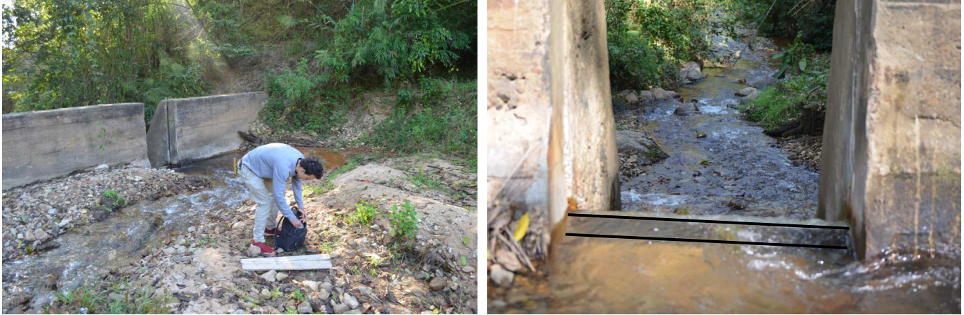
Figure 28: Rehbock weir 1, overview and zoom in after the installation of the weir. The weir can be seen as the dark brown color between the two black lines. The lower line is the bottom of the river and upper the weir crest. The weir was tightened between the concrete construction.
