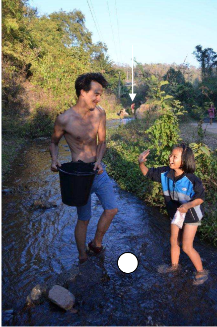
Figure 30: Injection point and measuring point of the slug tracer method. The circles represent the injection points and the arrows the measuring points.
