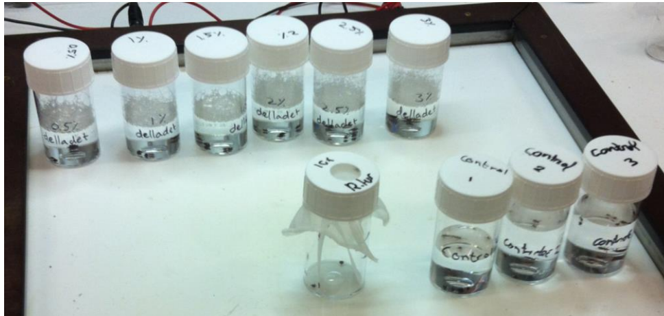
Figure 18. Experimental setup: 10 tubes; 1 without water (bottom-left), 3 tubes with only tap water (bottom right) and 6 tubes containing different Delladet concentrations (top).
