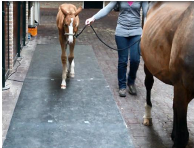
Figure 2. The pressure plate with the rubber mat and an example of a valid run.
