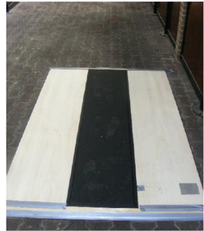
Figure 1. The setting of the pressure plate without the rubber mat.
