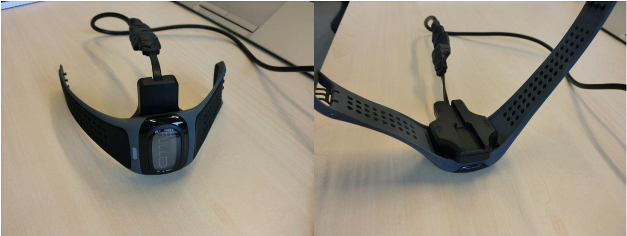
Figure 6 Photo of the MIO attached to the dongle, resting on its side or upside down
