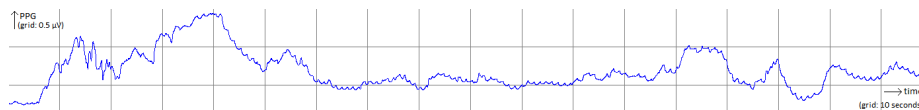
Figure 2.2: A sample PPG signal over 180 seconds, where the x-axis indicates the time passed, and the y-axis the amount of light absorbed by the skin.
