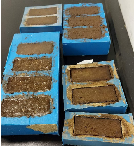
Figure 5: Samples created with a mixture of DS, gravel, NaOH, sodium silicate and Eco 2 cem.
