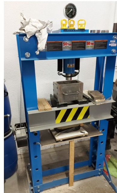
Figure 4: The hydraulic press that was used for the production of compressed samples
