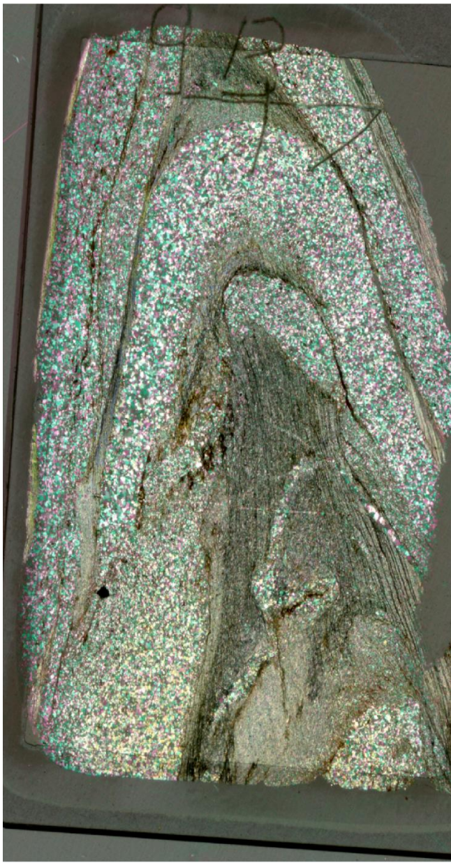
Figure 20. High-quality scan of thin-section 9B, showing a thinning of the pelitic layers in the flanks of the fold, while it is thickened in the hinge zones.
