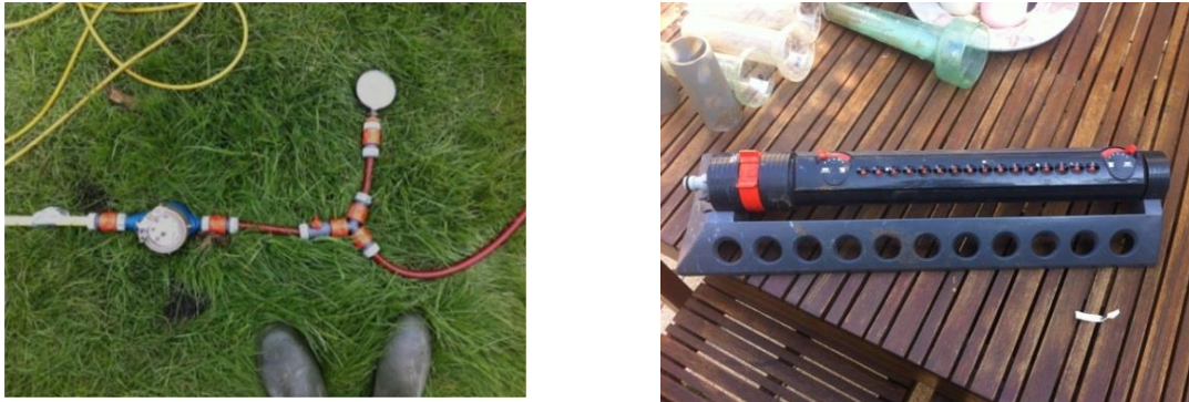
Fig. 4.2: (L) Photo of the connection between the flow meter, pressure adjuster and pressure meter, from left to right; (R) Photo the Gardena garden sprinkler.
