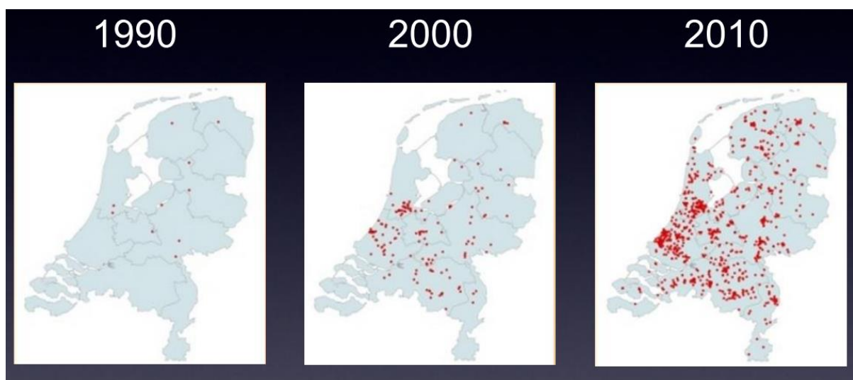
Figure 5 - ATES systems installed in the Netherlands (adapted from Worthington, 2012)
