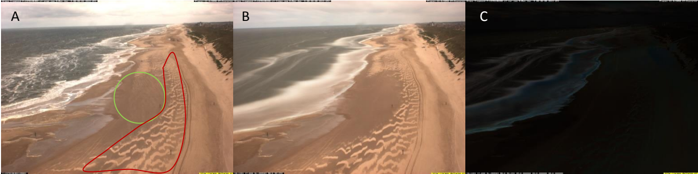
Figure 3.3: A Snapshot (A), time-exposure (B) and a variance image (C) from one of the cameras on top of the Coast3D tower at Egmond aan Zee. The red area indicates a zone with sand strips, the green circle an area with (hardly visible) streamers. Source: Argus Coast3D Tower.
