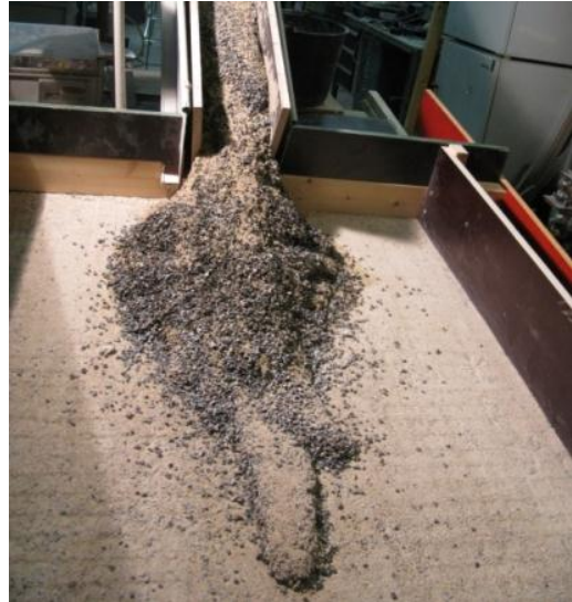
Figure 37: Photograph fan 1, 22 debris flows with 2x coarse material content (23.47wt%).
