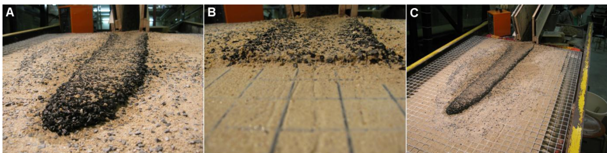
Figure 15: Photographs experiment 230 with 4x coarse material. A) coarse snout, B) cross-section coarse levees, C) overview.
