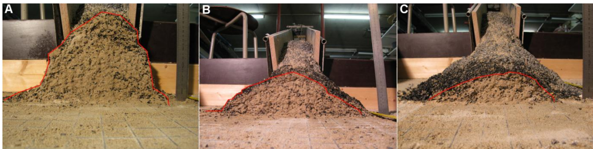
Figure 43: Cross-sections of fan 1 at 8, 24 and 44 cm from the apex.
