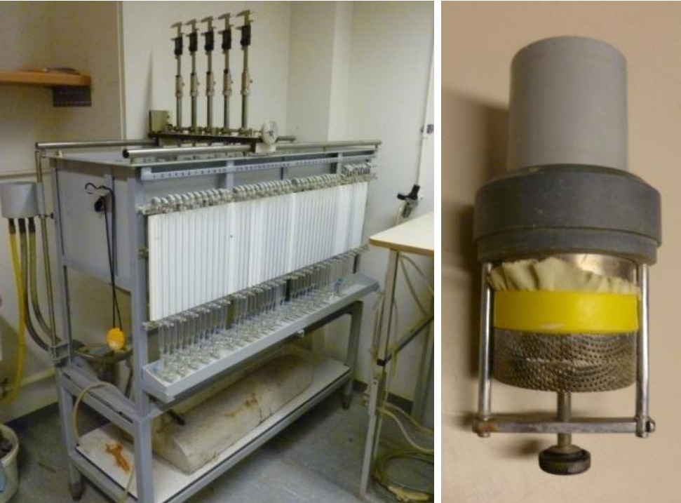
Figure 11: A) Permeameter. A water reservoir with a constant head. Burettes at the front and on top a system for measuring detailed water heights. B) Sample holder of the permeameter. Sample is covered with a gauze and a small metal raster.
