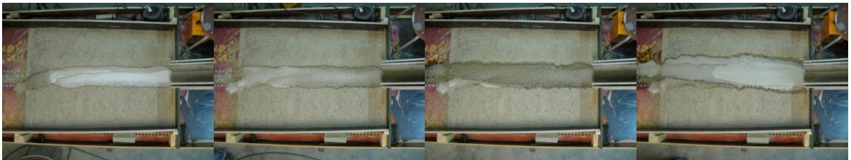
Figure 40: Top-view photographs of different steps in the formation of fan 1 after debris flows 2, 3, 4 and 6. Movie showing all top-view photographs ( http://youtu.be/C5SjM3lnZ0g ).
