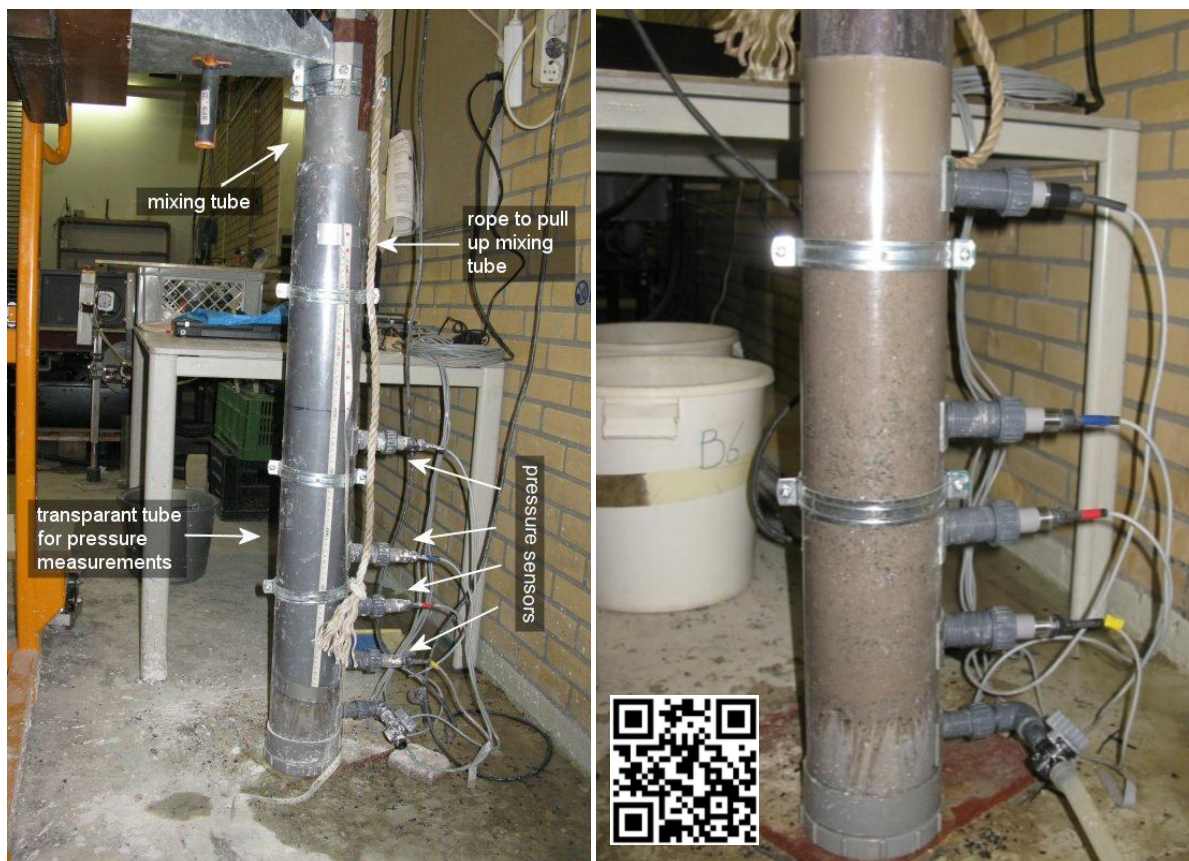
Figure 13: A) Setup of diffusivity experiment. B) Photograph experiment in progress and movie about diffusivity experiment. ( http://youtu.be/9XGQ75FAVYk ).
