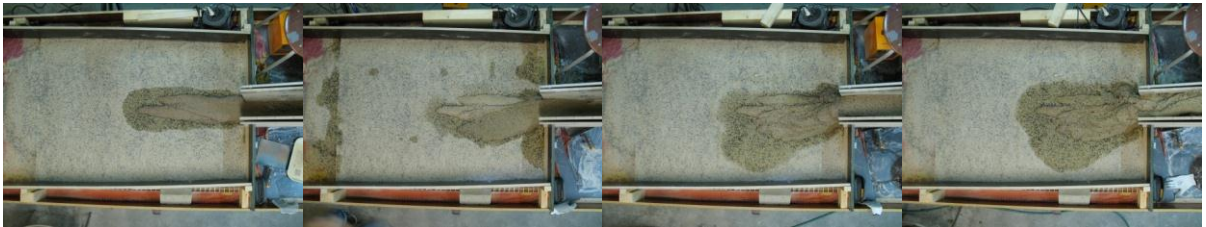
Figure 41: Top-view photographs of different steps in the formation of fan 1 after debris flows 2, 12 and 19. Movie showing all top-view photographs ( http://youtu.be/B_oqo4FnRHw ).
