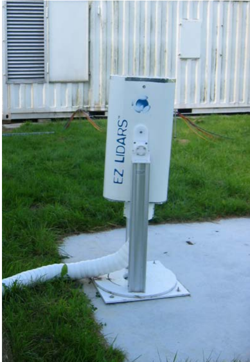
Figure 2.1. Picture of the LEOSPHERE ALS450 UV-lidar located at the remote measuring site of the Cabauw experimental site for atmospheric research (CESAR). This lidar operates at a wavelength of 355 nm with a temporal resolution of 30s and a vertical resolution of 15 meters.
