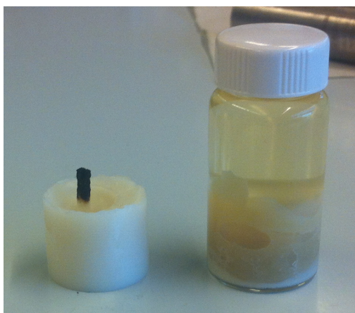
Figure 16. Image of waxes collected after FT synthesis for Co/SiO 2 (left) and Co/CNT (right) catalysts.
