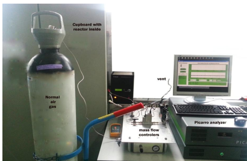
Figure 317: Experimental setup: normal air is flushed from the cylinder to the reactor inside the chamber, through the mass flow controllers. It leaves the reactor and ends up at the Picarro analyser.
