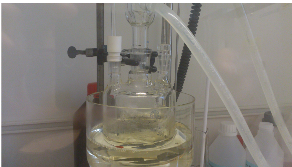
Figure 3.1: Set-up used for the esterification of silica substrates with stearyl alcohol in TEP.
