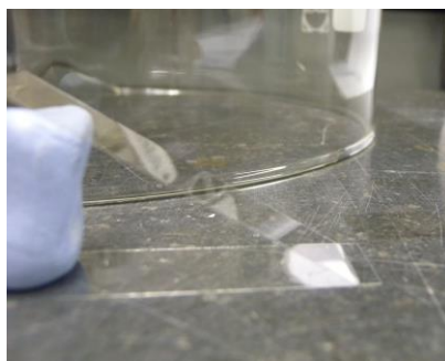
Figure 27: Setup used in a HD experiment with 1 %V fluorescent hollow silica cubes(HC_R_fIH) in water, showing a deposit was formed at the bottom slide
