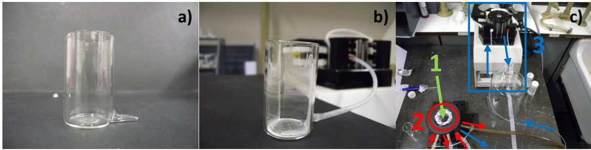
Figure 28: FCVD setup a) Specially designed glass flask used for FCVD experiments b) Flask after a FCVD experiment connected to a peristaltic pump, showing particles sedimented on the edges of the flask c) Complete setup of a FCVD experiment with 1. The sample 2. The construction of the thermostatic waterbath 3. The peristaltic pump
