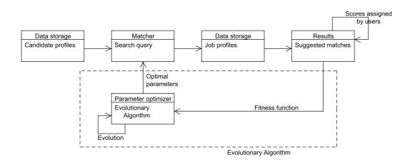
FIGURE 3.6: Architectural view of the parameter optimzer.
