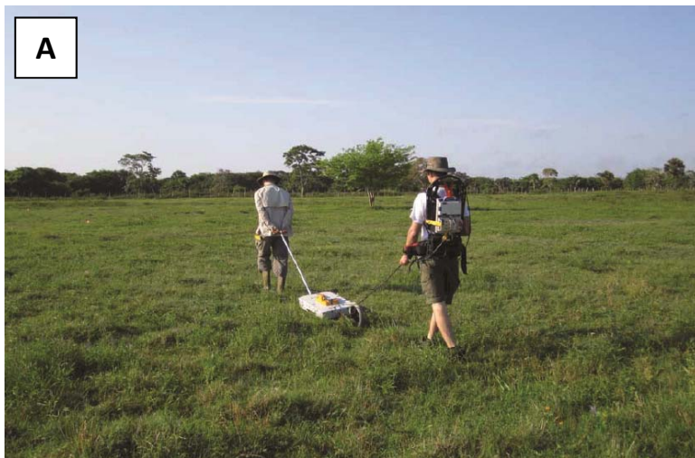
A: GPR measurements performed during the field campaign of 2012 (Photo: W.Z Hoek) and B: the basic principle behind the GPR method. C: the transect along with the GPR measurements were obtained and the multiple analyzing steps which were performed by R. van Dam
