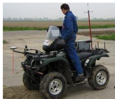
Figure 8: Farmers use RTK-GNSS equipment mounted on a quad (H-Wodka, 2010)
