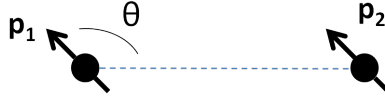
Fig. 3. Model of two rods as fixed parallel (mathematical) dipoles. The connecting line between the positions of the dipoles makes an angle \theta with the direction of the dipoles.
