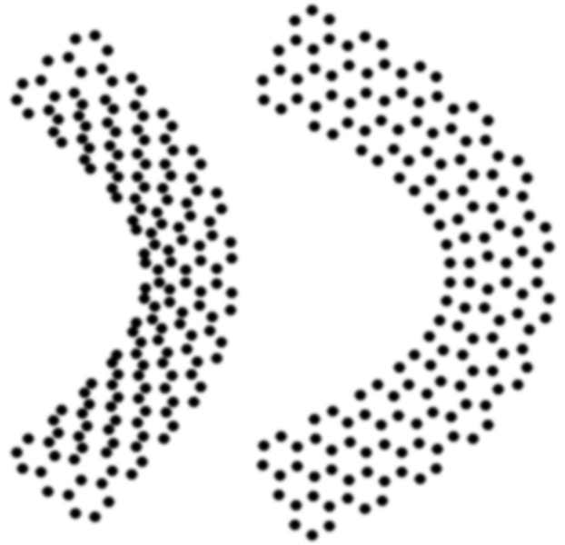
FIG. 2. Bending can be compensated by angles, bonds or a combination of the two. These rather extreme examples show the limiting scenarios, generated by performing a MM simulation with parameter ratios of 0.01 and 100 \text{ \AA}^{-2} \text{ rad}^{-2} respectively.
