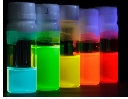
FIG. 2. A quantum dot rainbow. Each subsequent vial contains quantum dots with increasing particle size, decreasing HOMO-LUMO gap and increasing the fluorescence emission wavelength. Courtesy of prof. Andries Meijerink, Condensed Matter and Interfaces, Utrecht University.
