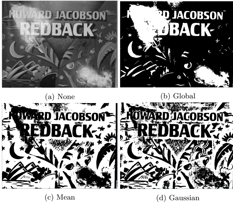
Figure 4.2: Different thresholds applied to the same image
