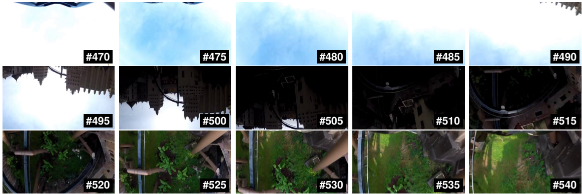
Figure 4.5: Frames 470-540 of a roller coaster video sequence (see Figure 4.6). Frames 478-486 are just shots of the sky, causing the edge detector to detect no edges. Frames 495-525 show the camera autocorrecting for illumination. At frame 538 (not shown here), a false positive is sometimes detected.
