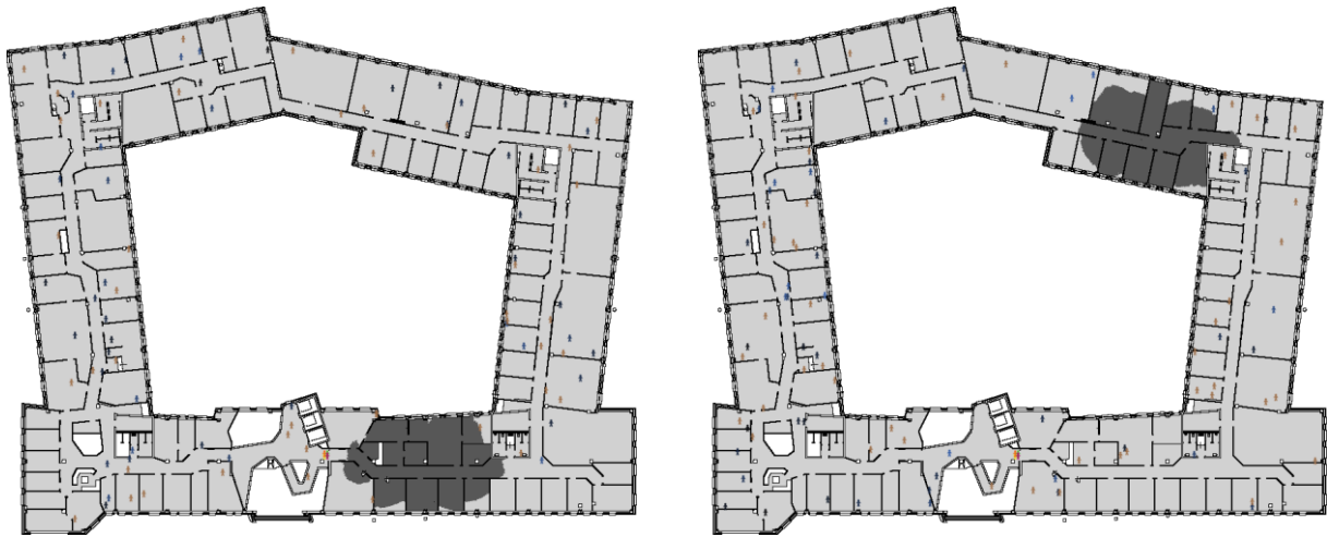
Figure 18 (on the left side) and figure 19 (on the right side): the smoke model implemented in the evacuation model; with the smoke on the bottom of figure 18 and on the top right side of figure 19.
