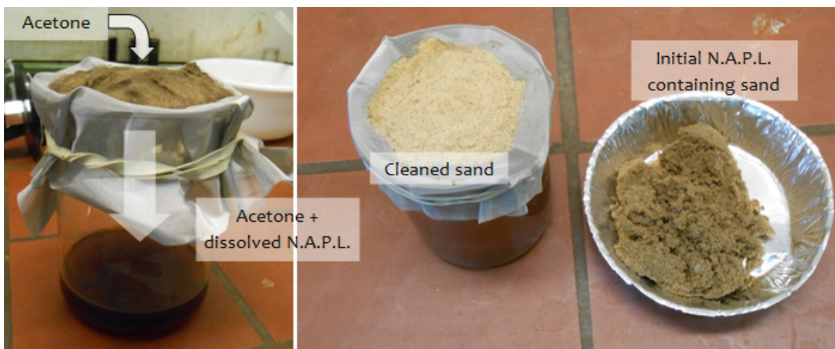
Figure 2.19: Sand cleaning procedure and result
