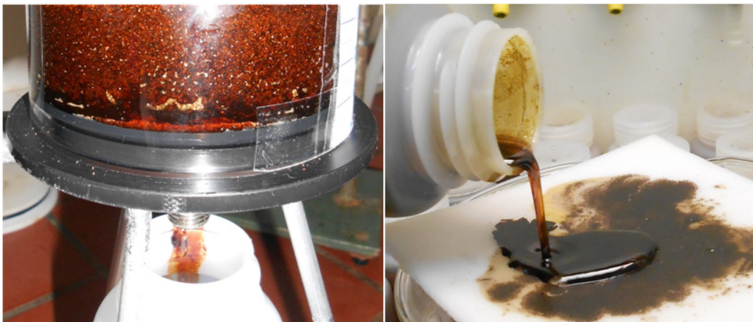
Figure 3.8: Mixed product right after NAPL breakthrough (left) and during NAPL-water separation process (right)
