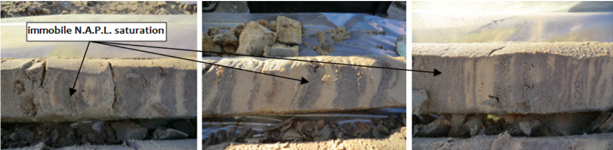
Figure 2.3: Representative sonic drilling cores containing immobile NAPL saturation [14][13]
