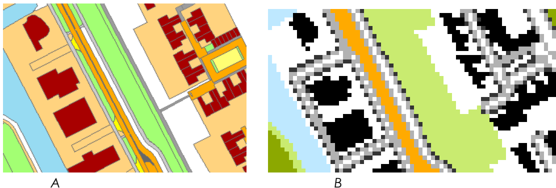
Figure 9: Example of a road with a cycle path in BGT (A) and TOP10NL (B)
