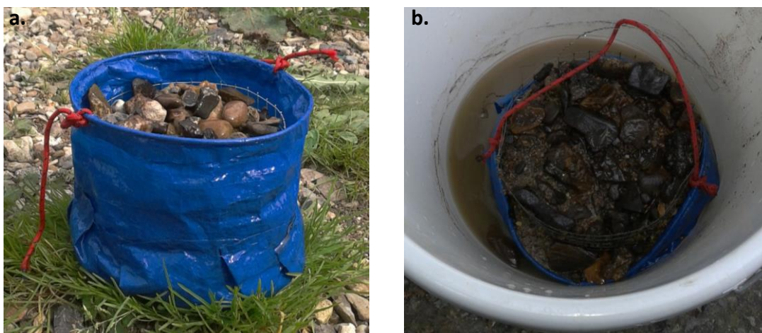
Figure 2. a) a trap before it is buried in the river bed, with the bag still pulled up. b) a trap that has just been removed from the river.
