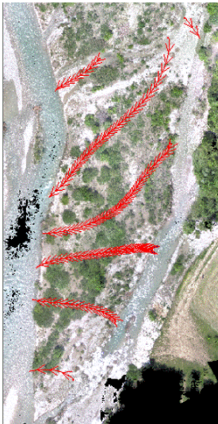
Figure 3.23: Flow paths of infiltrated water and solutes in the north-east. Every arrow represents a residence time of 10 days.
