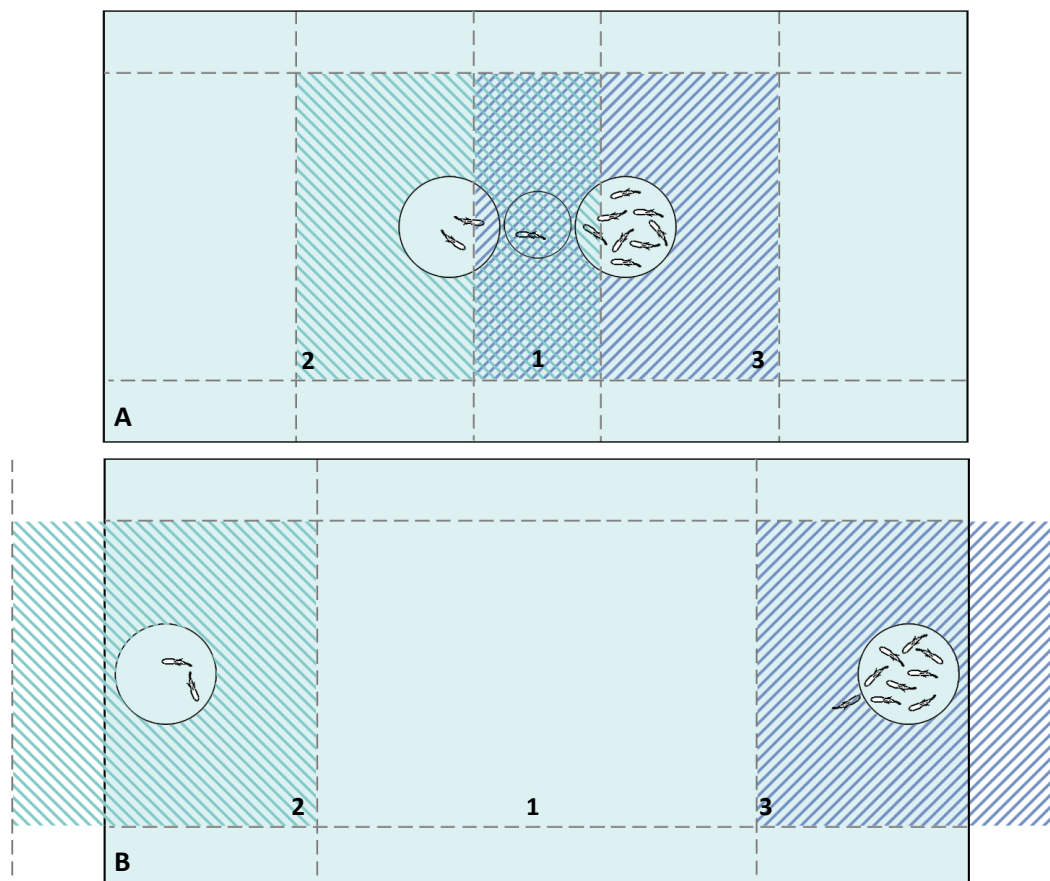
Figure 2. Schematic of the test tank with dynamic setup, setup B, as used in experiment 1. Plan view. Stimulus shoals are presented in two moveable, transparent plastic cylinders. Dashed lines mark the boundaries of both shoaling zones, which were marked by lines on the outside and at the bottom of of the tank, at 12 cm from the stimulus shoals. The diagonal lines mark both shoaling zones in the picture (2 and 3). 1 is the central compartment, in which the subject is released. 2A shows the situation at the start of the experiment, where the subject is still acclimatizing in a transparent plastic cylinder and both stimulus shoals are still near the center of the tank. Figure 2B shows the situation after the stimulus shoals have been moved towards the outer ends of
