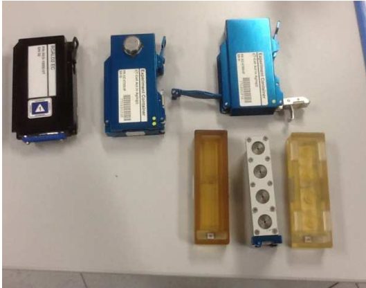
Figure 3: Different kinds of experiment containers. The lower right side illustrates an experiment that has to be 'activated'.
