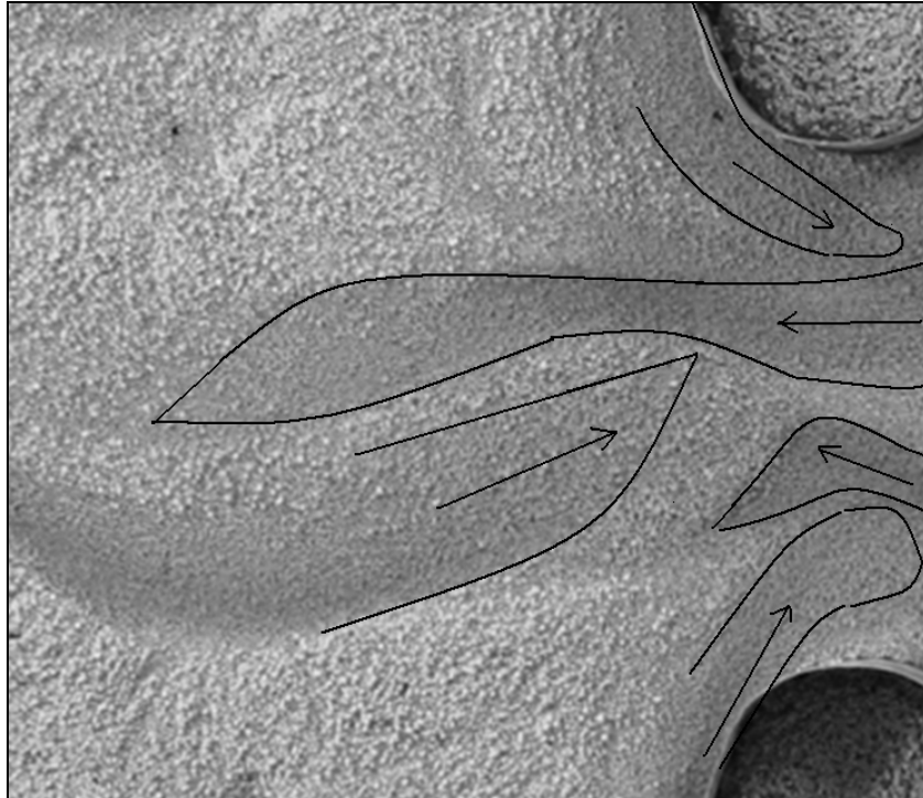
Figure 5.2 Image of final configuration in experiment 28 at low water. The sketch represents the “evasion” of flood and ebb channels typical for tidal channels as in figure 5.1. It proves alternation of flood and ebb transport during experiment 28.
