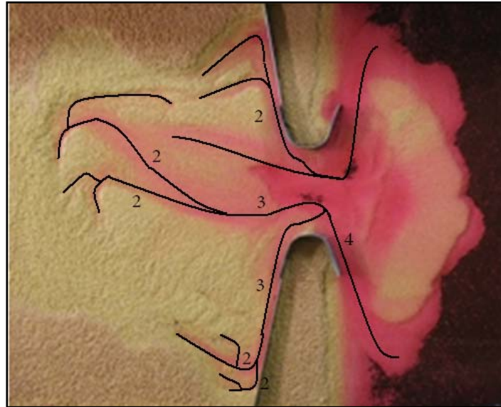
Figure 5.10 Experiment 29, photo 1842. According to Horton’s hierarchical analysis the system is a four-times branching network.
