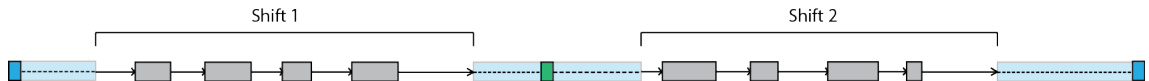
Figure 4.4: An example of a route with two shifts. The blue rectangles represent the start and end of the route, and therefore also the start of the first shift, and the end of the second shift. The green rectangle is a shift start action, this is where the first shift ends and the second shift begins. The solid arrows indicate travel time, whereas the dotted lines are waiting time. The transparent blue area indicates the use of the flexible duration of the depot actions. The duration of a depot action is stretched to remove all unnecessary waiting time. For example say we have a shift that is finished at 11:00 am, and a depot action that is scheduled to start at 12:00 am. The waiting time gap of one hour is then filled by extending the depot action to start at 11:00. The actual duration of the shift is indicated by the brackets on top of the representation.
